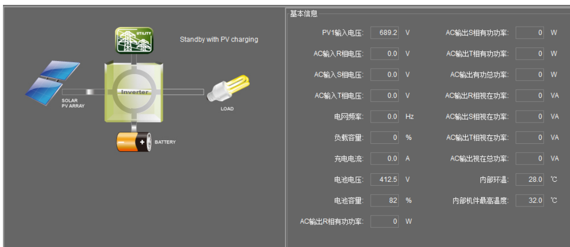
Fig3 in Standby with PV charging mode
