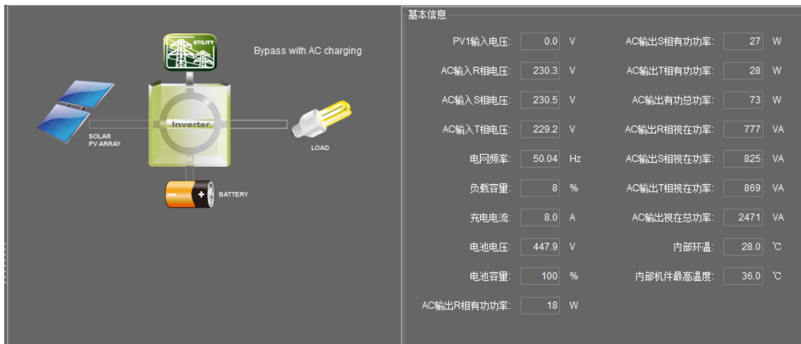
Fig2 in Bypass with AC charging Mode
